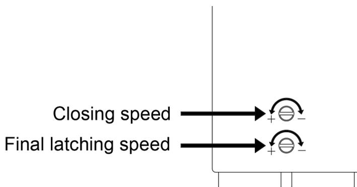
To adjust, turn both screws clockwise until they stop. This will mean the gate will be locked in position. Then undo until they are the correct speed ensuring they do not turn more than 3 full turns from the stopped position
